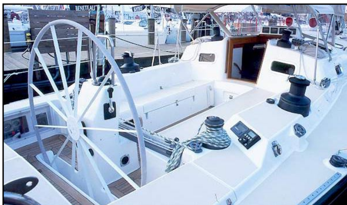
Edson Diamond Series wheel with "Comfort Grip" Leather Wheel Cover on a J-160.
